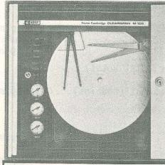
Electrical Controllers with mechanical or potentiometric measuring systems for most process variables. Four basic types of contact action with 23 varia-
